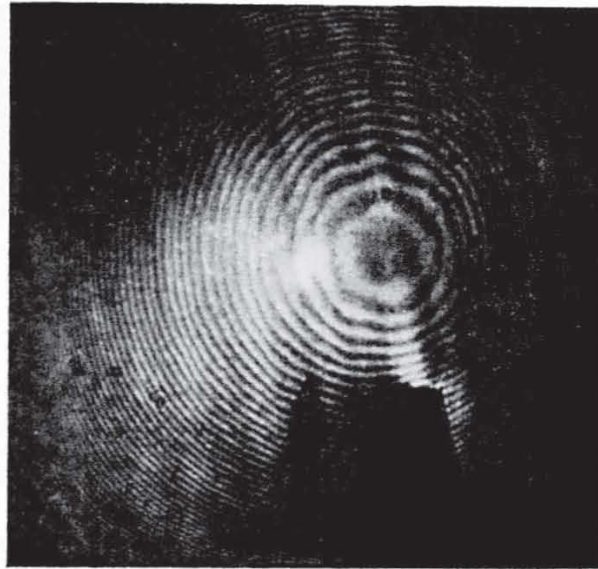
Fig. 10. Transient interference figure in a photoelastic arrangement with converging beams on a crystal immediately after switching off the applied field. The interference figure is the fan-shaped dark region from the upper left to the lower right. In the lower half a dark region originates from a crack that occurred in the crystal. The dominant interference ring system results from interference between front and back surface as in fig. 6.
