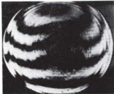
Fig. 7a: Interference pattern obtained from an aspheric Ge-lens surface manufactured by diamond-turning, tested with \lambda = 633 \text{ nm}
