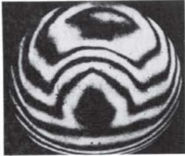
Fig. 6a: Interference pattern obtained from an aspheric surface from a glass lens tested with \lambda = 633 \text{ nm}
