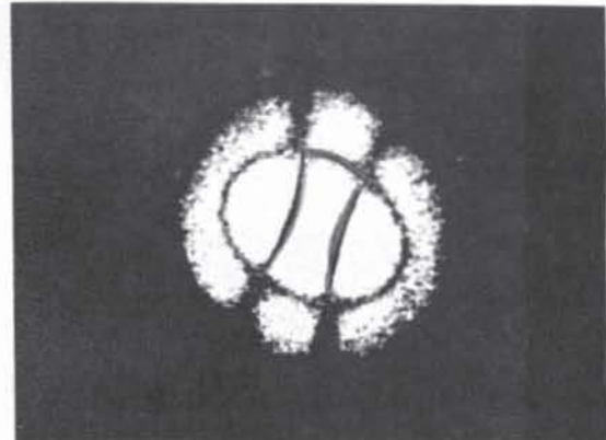
Fig. 15a: Quasi real time fringe pattern obtained in the time average, with BSO, of a harmonically oscillating membrane
