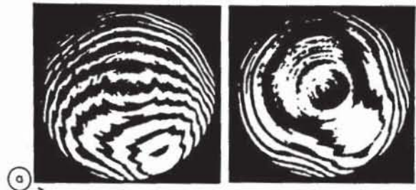
Fig. 2a: Interference pattern obtained from a diamond turned spherical surface tested with \lambda = 633 \text{ nm} .
