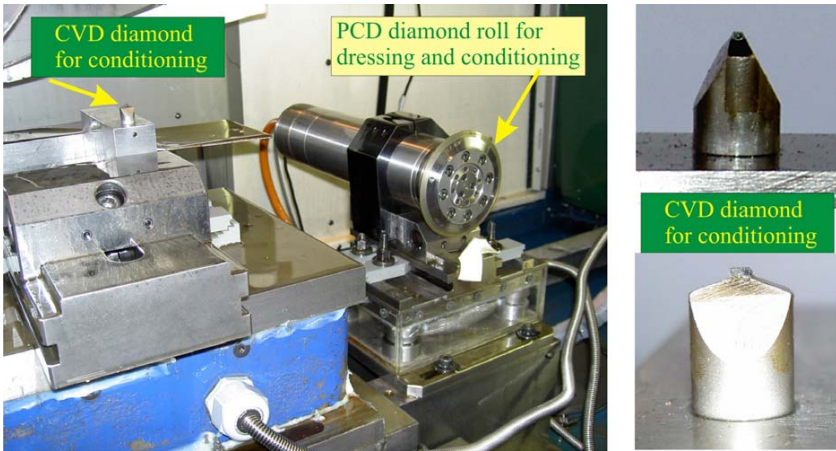
Figure 4.2: The two types of dressing tools used for wheel conditioning; a) CVD stationary tool, and b) PCD rotary diamond wheel
