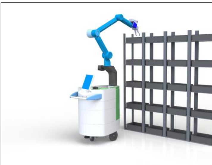
Figure 8.2-2 Design sketch for care utensil service robot
