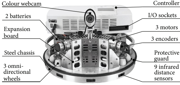
FIGURE 1: Festo Robotino and its main components (photo from Robotino manual [12]).
