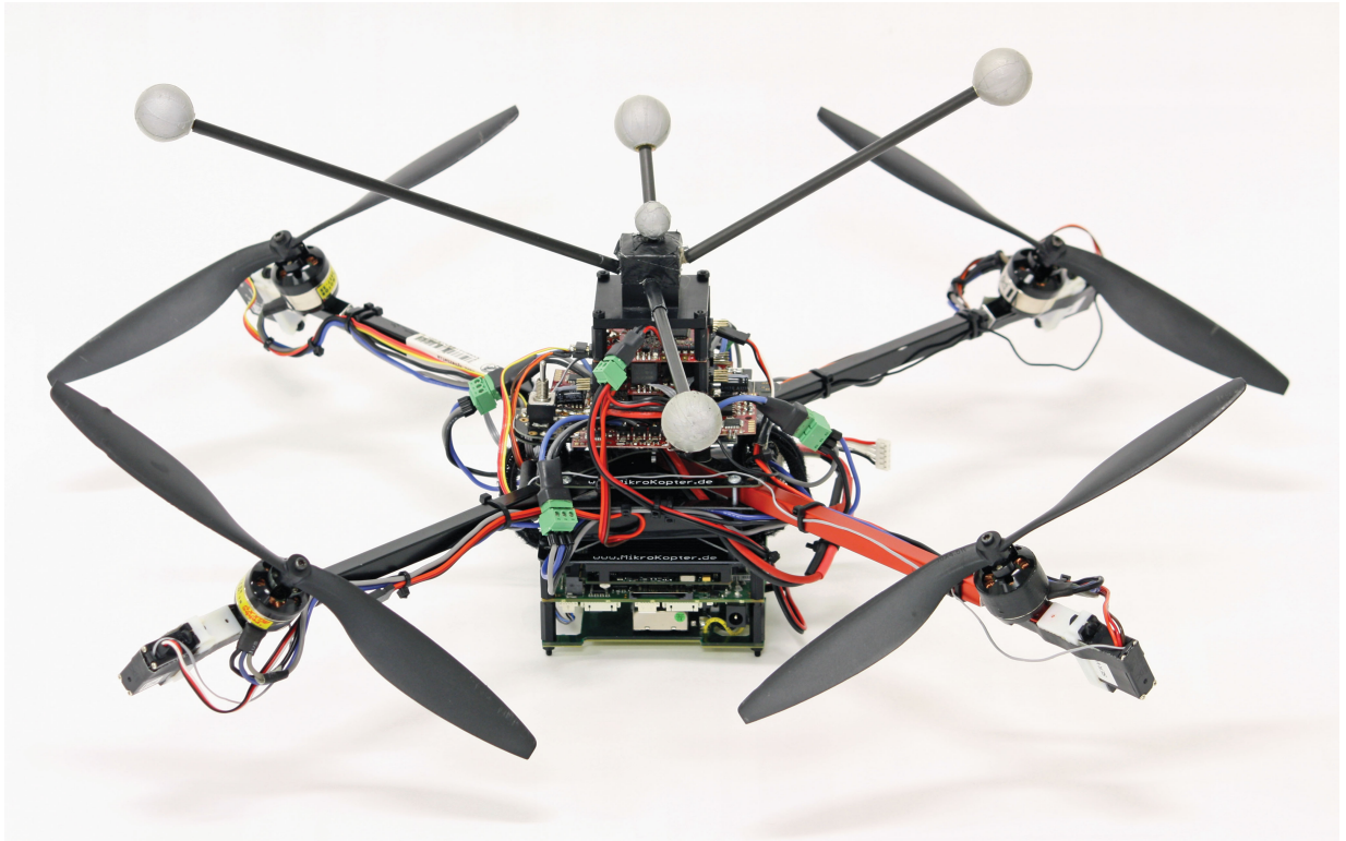
Figure 1.2: Picture of the holocopter prototype. The four propeller groups are slightly tilted. The red bar indicates the positive direction of the \mathbf{X}_B holocopter body axis
