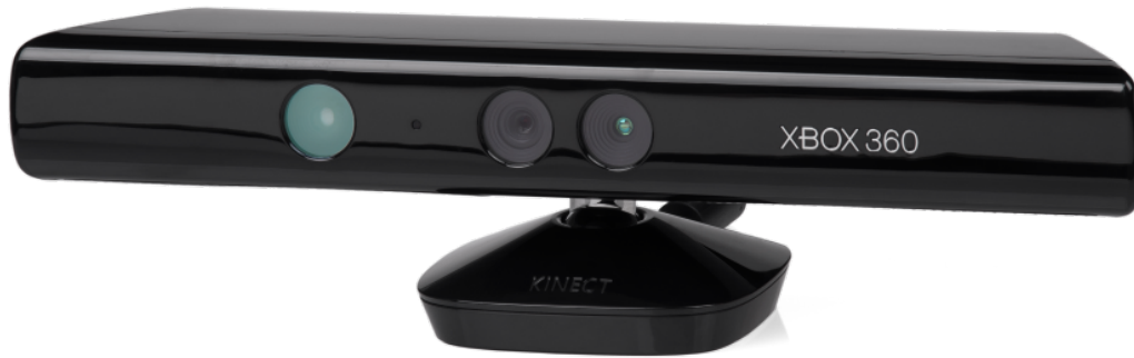
Figure 5: The Microsoft Kinect camera. A low cost depth sensor, initially intended as gaming input device, but grown into a very popular tool for research and engineering
