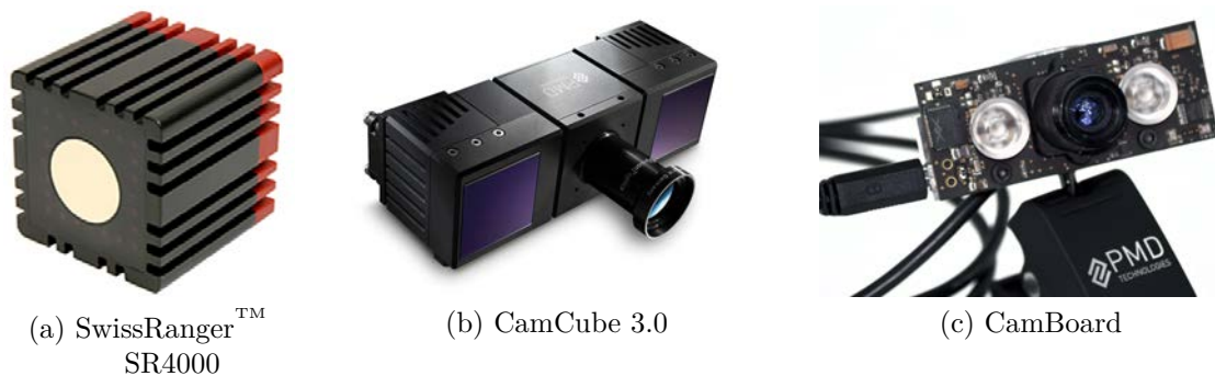
Figure 2.4.: Range imaging sensors based on the ToF principle manufactured by MESA Imaging and PMD[vision] ® .
