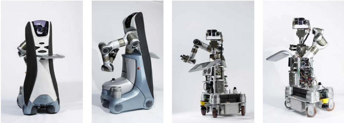
Figure 3.1.: Hardware design of the service robot Care-O-bot ® 3. The first two images show the robot's cover. It is flexible in the range of the torso to allow the robot to express itself by gestures. The other images show the robot's hardware design below the cover.
