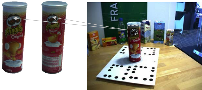
Figure 5.7.: Multi-occurrences of feature point p on a single object. A single feature point is associated to two different locations on the object image.
