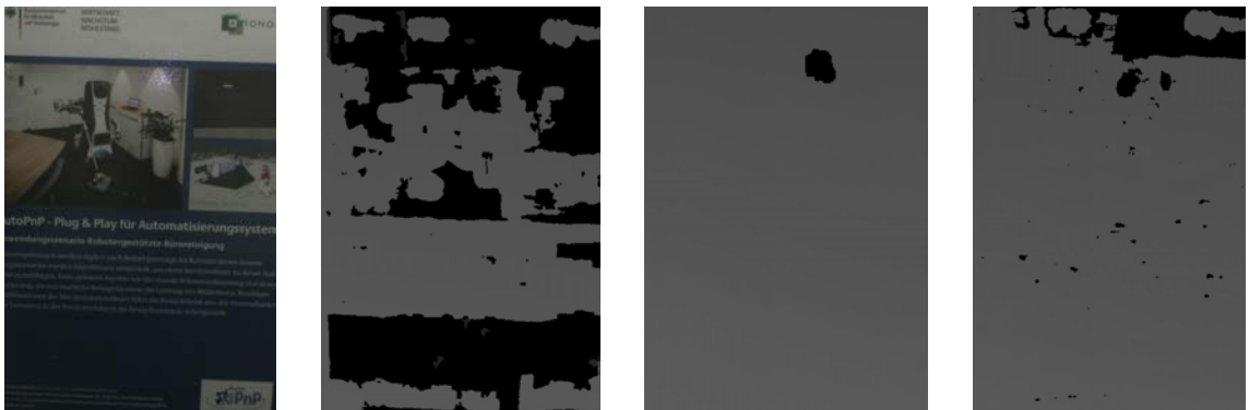
Figure 4.6.: Images of a planar surface: the original color image (first column), disparity from passive stereo vision (second column), disparity from the Microsoft ® Kinect ™ sensor (third column), and disparity from the proposed sensor combination algorithm (forth column).
