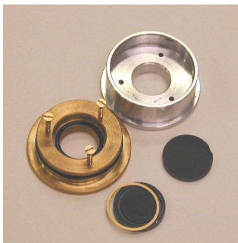
Fig. 3.4 The transmission cell. The two silicon plates (the dark discs in the image) are mounted inside the metal support, which closes with three screws. The cell is placed in front of the beam.
