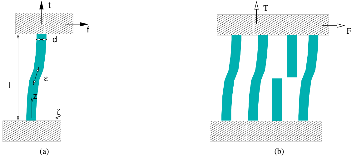
Figure 3.1: (a) Shearing of a single beam between two rigid plates. Since the distance l between the plates is kept constant, the beam experiences stretching and bending deformation, with longitudinal t and shear f forces. (b) Shearing of an array of beams, with the corresponding forces. In the case shown, one beam is broken.
