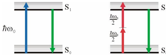
Figure 5.2. Comparison between one- and two photon absorption processes.
