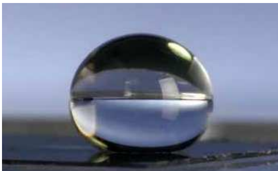
Fig. 1.1: Droplet on a superhydrophobic surface [1]. The substrate is covered by aligned, coated nanofibres. Here a droplet with a diameter of 2 mm resides on the tips of the fibres. The diameter and length of these fibres can be varied between 10–40 nm and 70–360 nm, respectively. The property of the surface can range between superhydrophobic and superhydrophilic depending on the type of coating.
