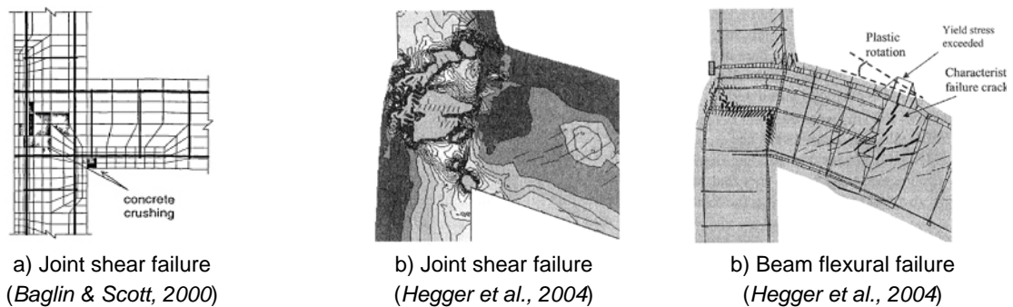
Figure 2-11: Simulations of monotonic tests on exterior beam-column joints
