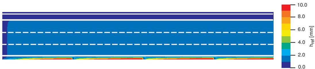
Figure 6.14.: Two dimensional water depth distribution for the modelled road section with  $a_d = 39$  m calculated with the Pavement Surface Runoff Model.
