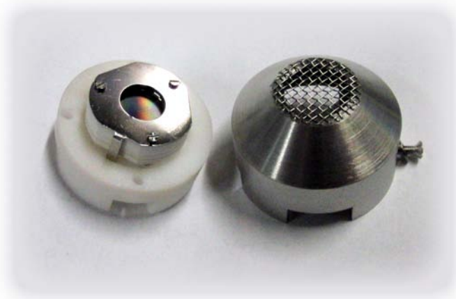
Figure 5.5 | Micro-channel plate and shielding cage. Photograph of the micro-channel plate detector (left) and the dismounted metal cage (right) that normally shields the high voltage at the MCP front side. The holder for the MCP is machined from Macor® glass ceramic.
