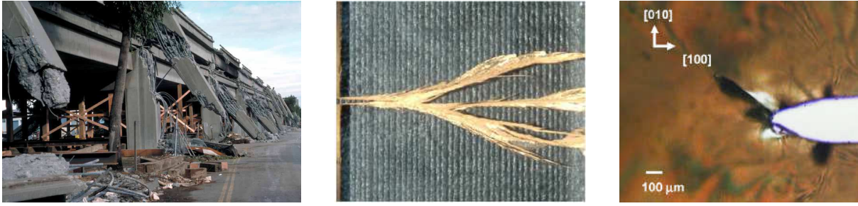
Figure 1.4: Illustration of materials at failure. Left: Bridge collapsing under an earthquake excitation. Center: Crack branching observed in brittle materials at dynamic loading. Right: Fracture in advanced electromechanical coupled materials.
