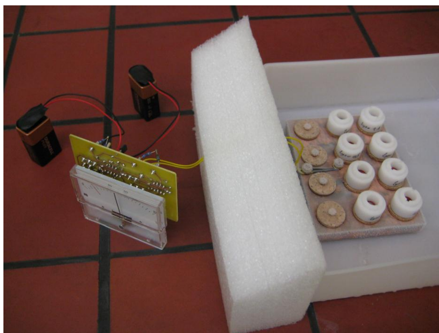
Fig. 3.16: The white sample preparation holders on top of the final version of the copper block with insulating cork discs and small tips. A vacuum tight thermometer attached to a PT-100 temperature sensor is seen on the left also important for the temperature control in the following lyophilization process. The cooling rate was manually varied by liquid nitrogen.
