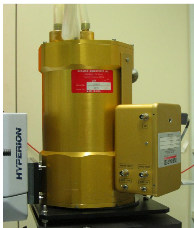
Fig. 3.5: The helium cooled bolometer which is used for far-infrared measurements.
