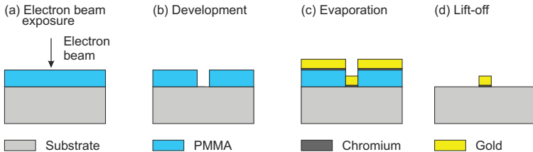
Figure 12: The individual steps to fabricate plasmonic nanostructures with EBL are shown. The exposure (a) is followed by (b) development. (c) A thin adhesion layer of chromium is evaporated before the gold. (d) Final lift-off dissolves the unexposed resist with gold on top and the nanostructure is obtained.
