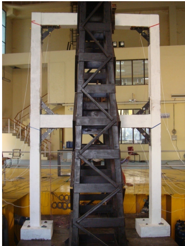
Figure 11.3 Layout of retrofitted structure on Shake Table
