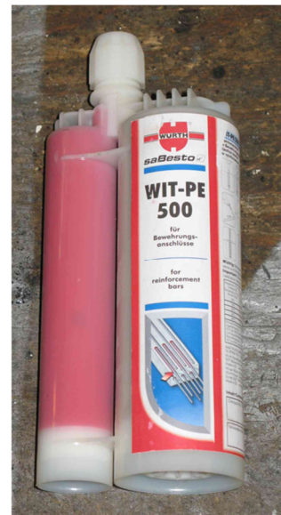
(b) Epoxy based Mortar
