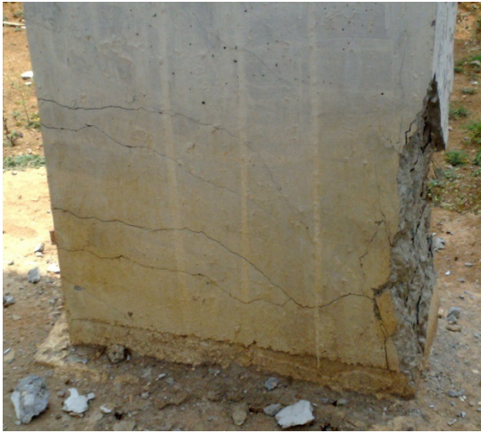
(a) CL 16 (Flexure-Compression)
