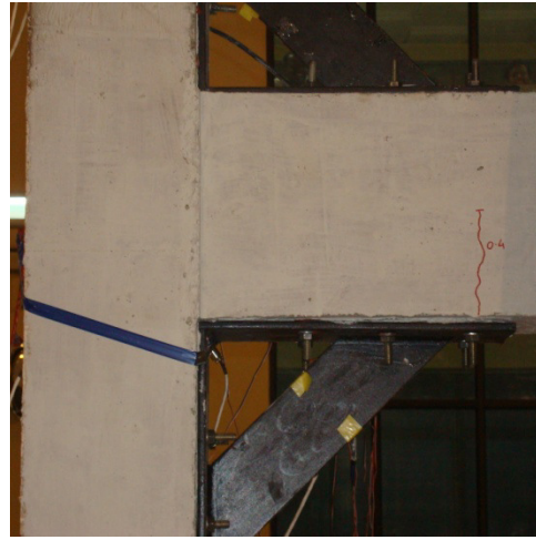
(a) At the base of left Side Column (b) On the beam of first floor (left side joint) Figure 11.15 Crack patterns observed after the base excitation of 0.4g
