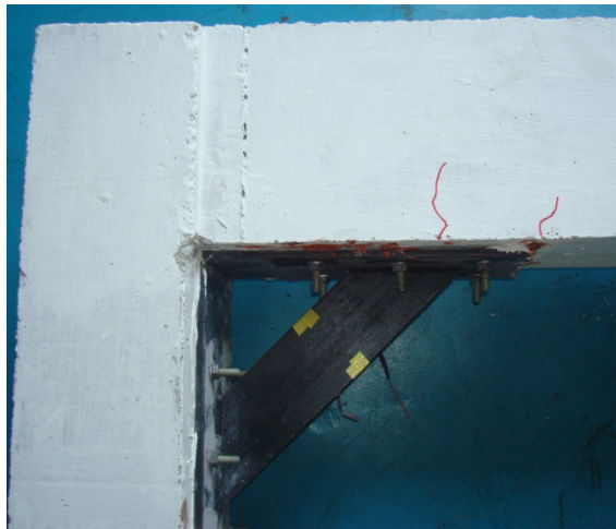
(a) Crack pattern for the left corner joint (b) Crack pattern for the right corner joint Figure 11.34 Crack patterns observed at the roof level for the retrofitted after the completion of test series
