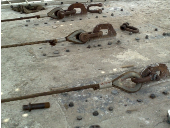
Figure 8.13 Loading arrangement at 3 rd floor slab
