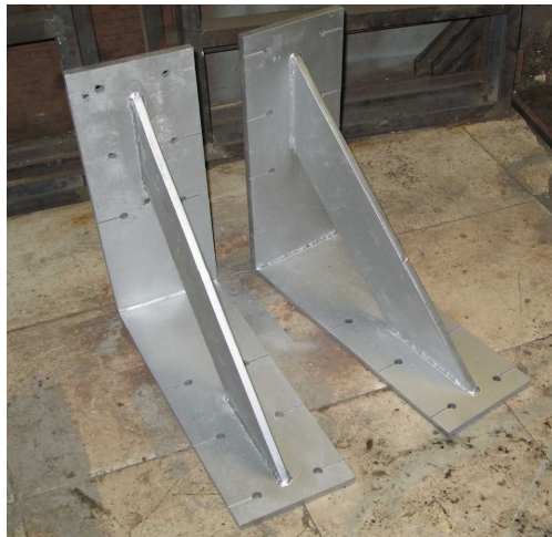
Figure 10.2 Fabricated haunch elements
