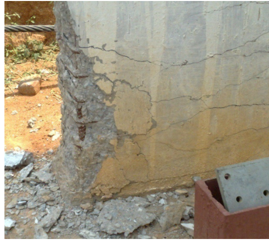
(b) CL 20 (Flexure-Compression)
