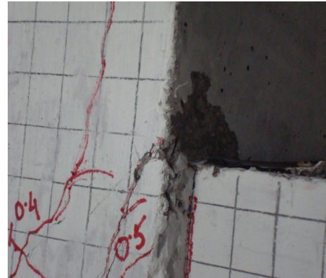
(a) Opened diagonal shear cracks in the joint panel (b) Spalling at top face of beam
