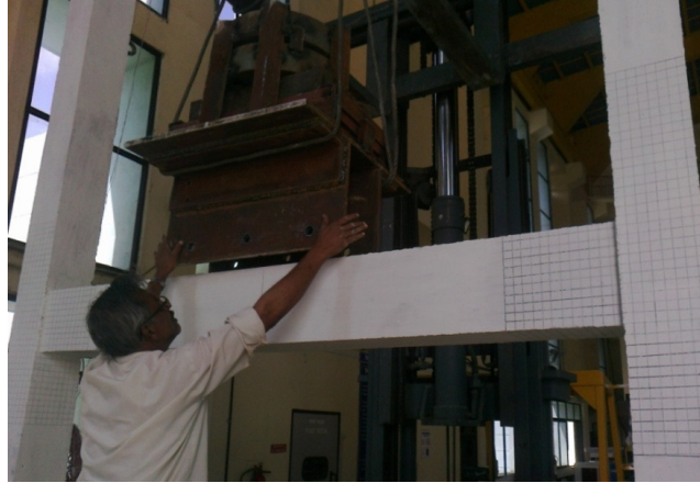
Figure 9.6 Added mass being placed on the structure
