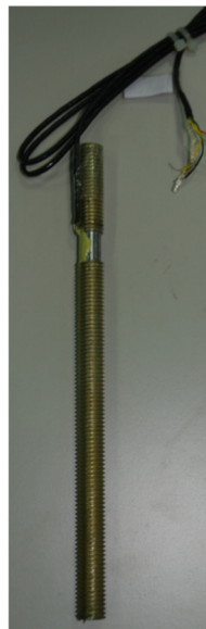
(a) Threaded rods with applied strain gauge
