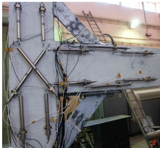
Figure 10.7 Potentiometer arrangement for retrofitted joint
