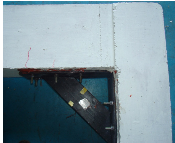
(a) Crack pattern for the left corner joint (b) Crack pattern for the right corner joint Figure 11.34 Crack patterns observed at the roof level for the retrofitted after the completion of test series
