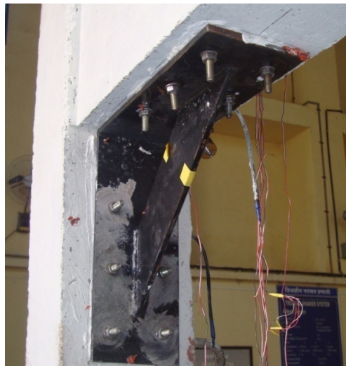
Figure 11.2 Haunch element installed using bonded anchors
