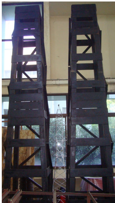
Figure 9.5 Support structures to prevent out of plane movement
