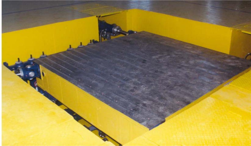
Figure 9.4 3D Shake Table at CPRI Bangalore
