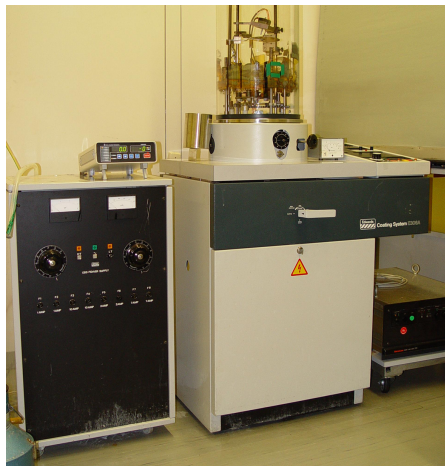
Figure 3.13: The evaporator Edwards E306.
