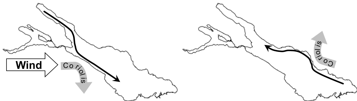
Figure 3.15: Conceptual sketch of surface currents during (left) and after the wind event.
