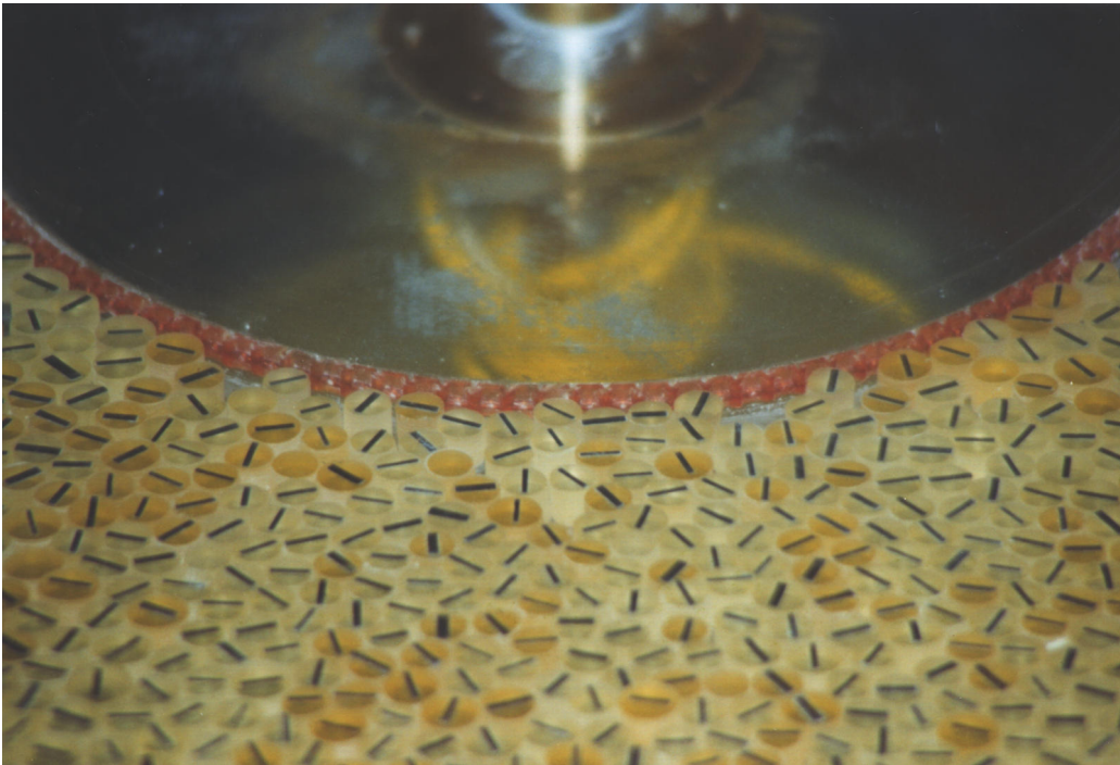
Fig. 3.1: Plexiglas disks near the inner shearing wheel of the Couette shear device of the Behringer group. (Photo: USA, Durham, 1999, Marc Lätzel)
