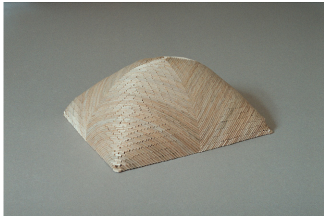
Figure 4 Model of complete vault; note the rather long courses in the lower and central regions (Wendland 2007).
