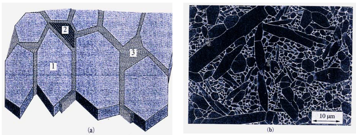
Fig. 2.8 : Typical microstructure of a liquid-phase sintered \text{Si}_3\text{N}_4 ceramics [schematic (a) and SEM micrograph (b)].
