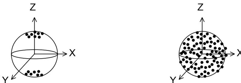
Figure 6.3: Pole sphere figure representation of highly oriented and completely unoriented material
