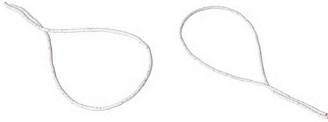
Figure 21.2.: Self-folding of carbon nanotubes. Our simulation results suggest that the folded state is in thermodynamical equilibrium at low temperature and unfolds at a critical elevated temperature [37].
