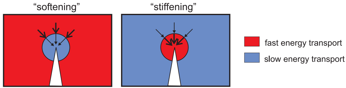
Figure 8.6.: The effect of a soft and stiff zone near the crack tip on the energy flux. In softening materials, energy flux at the crack tip is reduced due to reduced local wave speeds. In contrast, energy flux is enhanced in the vicinity of the crack tip in stiffening materials.
