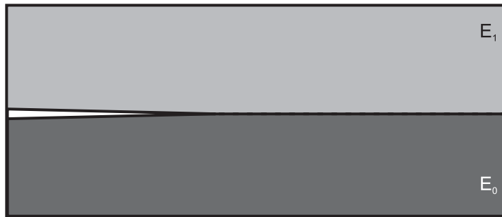
Figure 9.1.: Geometry of the simulations of cracks at bimaterial interfaces.
