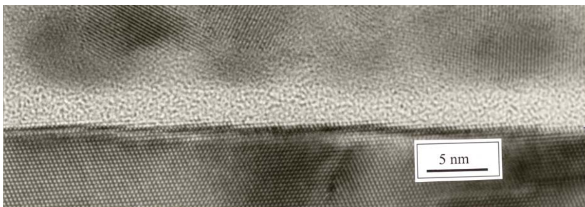
Fig. 3.13 TEM micrograph of a film annealed at 450 °C for 4 h, after initial deposition on Si wafers modified by mercapto-terminated SAM with hydrocarbon molecules consisting of only three carbon atoms from a solution containing 100 mM [Zn], 4000 ppm copolymer and 7 mM HMTA at 80 °C for 4.5 h.
