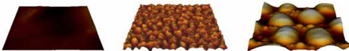
Figure 5.1 The 3D height profile (10 \mu\text{m} x 10 \mu\text{m} , z-range: 0 nm [dark] - 580 nm [bright]) of surfaces 1, 5, and 9 as measured by AFM in contact mode.
