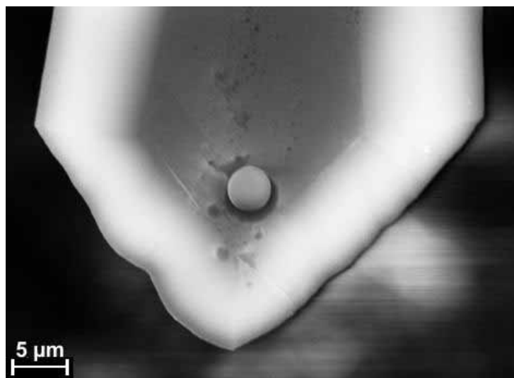
Figure 3.4 Gluing of inorganic particles to AFM cantilevers is well known in the AFM community. Here a Si sphere was attached to a tipless cantilever to investigate size effects in adhesion measurements 79 .
