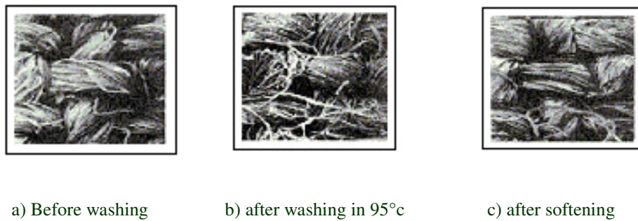
Fig 7. Effect of the washing and softening on the surface of a knitted fabric
