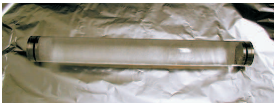
Figure 4.4: Photo of an ice single crystal inside the plastic tube in which it was grown.
