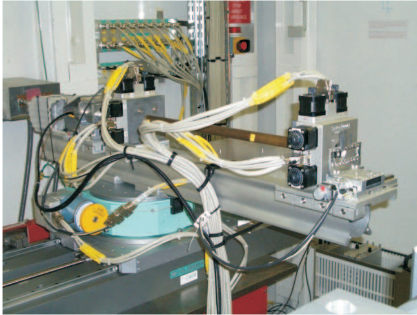
Figure 4.15: View of the detector arm. The detector elements are mounted on a X-95 rail. The lower part of the picture shows the rotation stage and the linear translation, which are combined to mimic the horizontal scattering angle.
