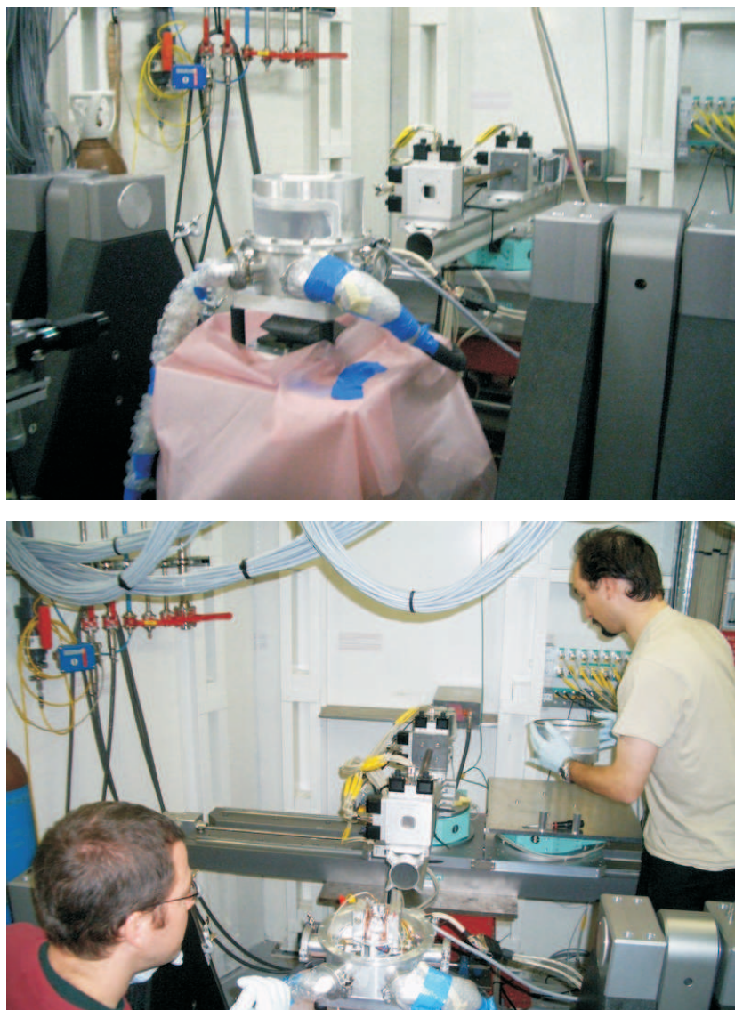
Figure 5.1: Photos of the experimental setup during the beamtime June 2005. The peltier cooling chamber is mounted on the diffractometer. Top: Setup during the measurements. Bottom: Setup during sample change. The sample is wrapped in aluminum foil to prevent ice sublimation. It is clamped between the copper plates in the center of the chamber.
