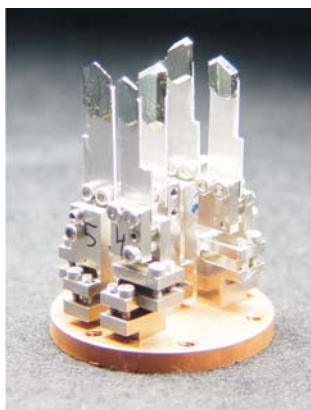
Figure 6.6: (a) Mosaic crystal array (Mosaic) of five single NbSe_2 crystals co aligned each on a single tiny goniometer [119]. The diameter of the copper disc is 4cm . (b) Larmor diffraction from the (201) Bragg peak of the mosaic samples. The data represents multiple Gaussians coming from different crystals. The mosaic spread of each single crystal is estimated to be 4' and the effective mosaic spread of the whole sample 10'
