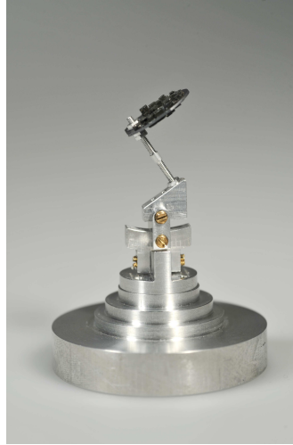
Figure 2.20: Sample with crystals in aluminum plate mounted on a multi-goniometer holder
