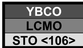
Figure 7.11: Structure of a bilayer consisting of 50 nm LCMO grown on vicinal cut STO and covered with a layer of 100 nm YBCO.
