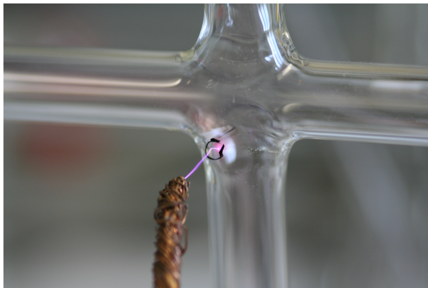
Figure 6.4: Microleakage in glass easily visible with the spark-vacuum tester under dynamic vacuum.
