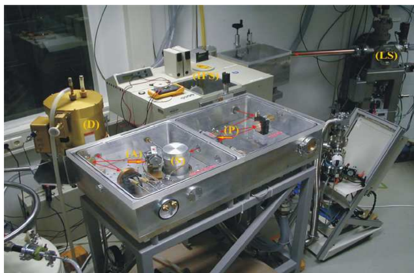
Figure 4.4.2 Infrared spectroscopic ellipsometry setup installed at ANKA beamline, Forschungszentrum Karlsruhe. In the extreme FIR – FIR region synchrotron radiation is used. For the MIR range conventional light sources are available. (LS) – the beam line, (IFS) – infrared FT spectrometer, (P) polarizer, (S) – sample cryostat, (A) – analyzer, (D) – LHe bolometer detector.
