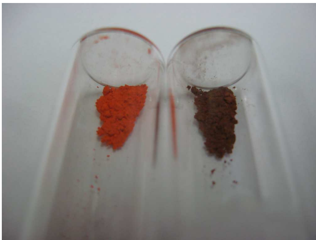
Fig. 3.37: Brown colour of \text{Pb}_3\text{O}_4\text{F}_x (right) versus orange colour of pure \text{Pb}_3\text{O}_4 (left)
