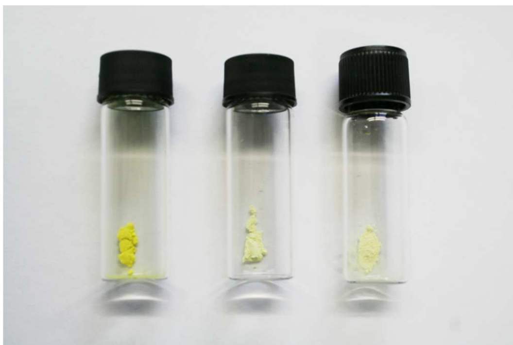
Fig. 3.16: Samples of HP- \text{Bi}_2\text{O}_3 (left), R- \text{Bi}_2\text{O}_3 (middle) and \alpha - \text{Bi}_2\text{O}_3 (right)
