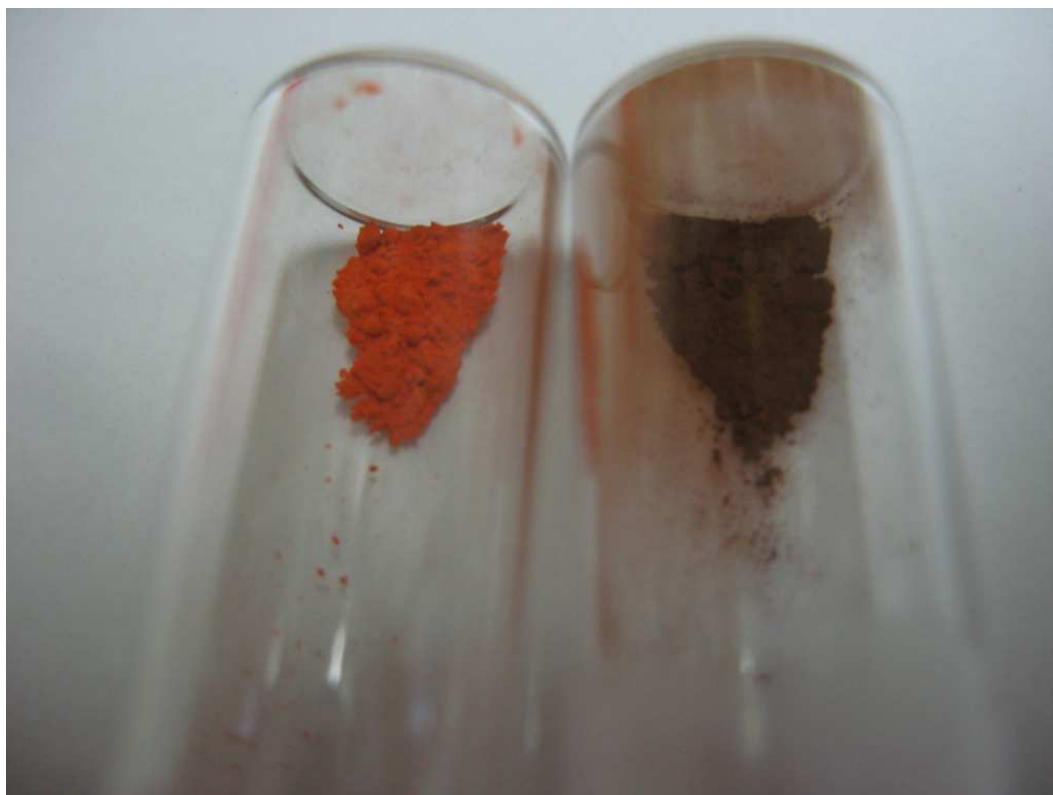
Fig. 3.43: Brown colour of \text{Li}_x\text{Pb}_3\text{O}_4 (right) versus orange colour of pure \text{Pb}_3\text{O}_4 (left)
