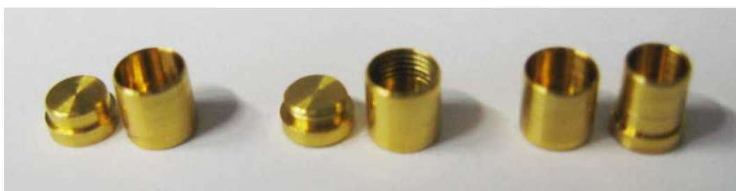
Fig. 2.11: Au capsule (width: 4 mm) in 3 designs: 'plain' (left), 'screw cap' (centre) and 'double cup' (right)
