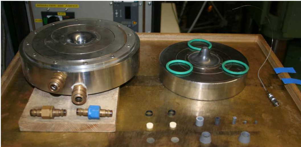
Fig. 2.6: The two matrices of the belt press module along with pressure cell components (displayed in the foreground)
