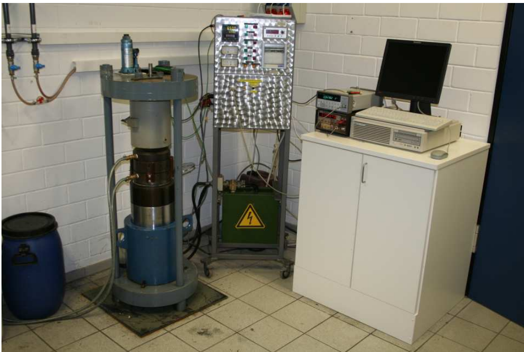
Fig. 2.2: The piston-cylinder press used in this work
