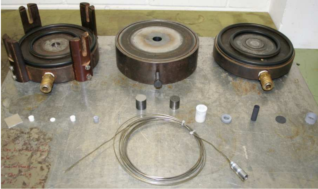
Fig. 2.3: The three matrices of the piston-cylinder press module, along with the pressure cell components (displayed in the foreground)
