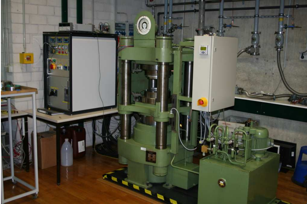
Fig. 2.5: The belt press used in this work (refurbished, with state-of-the-art electronic control panel)
