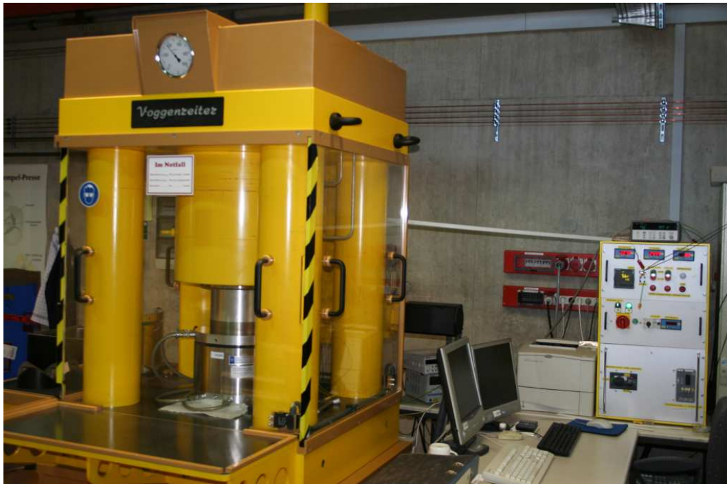
Fig. 2.8: The multi-anvil press used in this work
