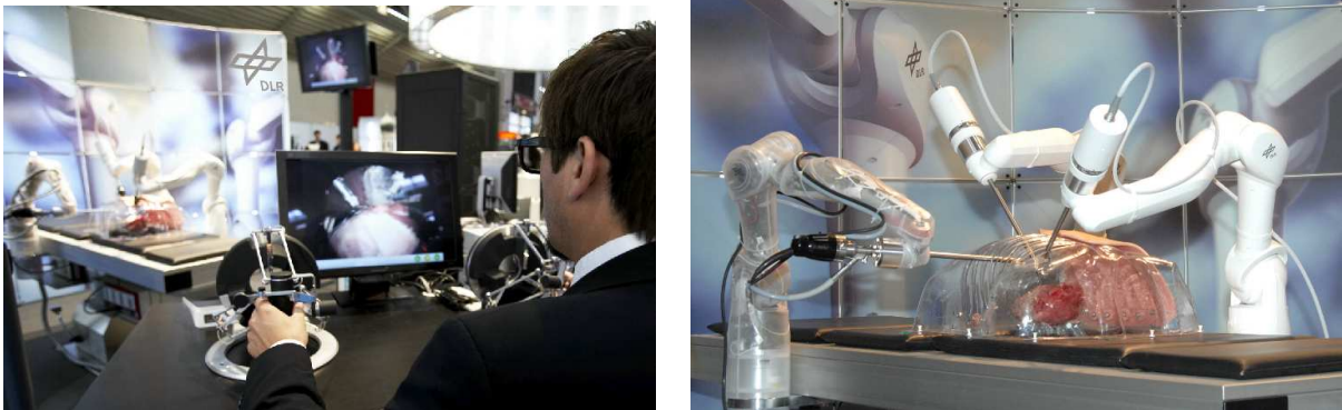
Fig. 1.1: DLR surgery scenario. Left: remote surgeon with force feedback input devices and 3D display. Right: DLR slave system consisting of three MIRO robot arms; one carrying the endoscope (semitransparent), two more carrying MIRS instruments for two handed manipulation (photos: DLR).
