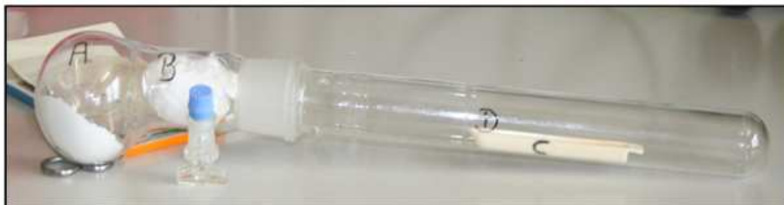
Fig. 3.3. The Drying Gun. ( Trockenpistole ) A ) Glass round bottom flask with the dessicant / drying agent (Sicapent with indicator). B ) Cotton ball for preventing turbulence and to prevent the worst case of mixing the two substances during evacuation. C ) Corundum crucible (boat) containing substance to be dried. D ) Round glass test tube to be placed finally in the furnace.
