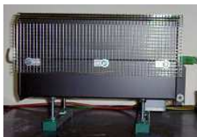
Figure 2.5: Single zone furnace (HTM Reetz GmbH, Berlin) used for synthesis in present this study.
