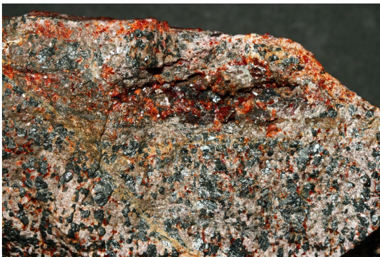
Figure 9.1: Zincite mineral (ZnO) from Franklin Hill Mine in New Jersey, USA - The picture shows the vein "in situ" in the granular ore of zincite. The mineral size is 8 x 5.3 cm 2 . [256]
