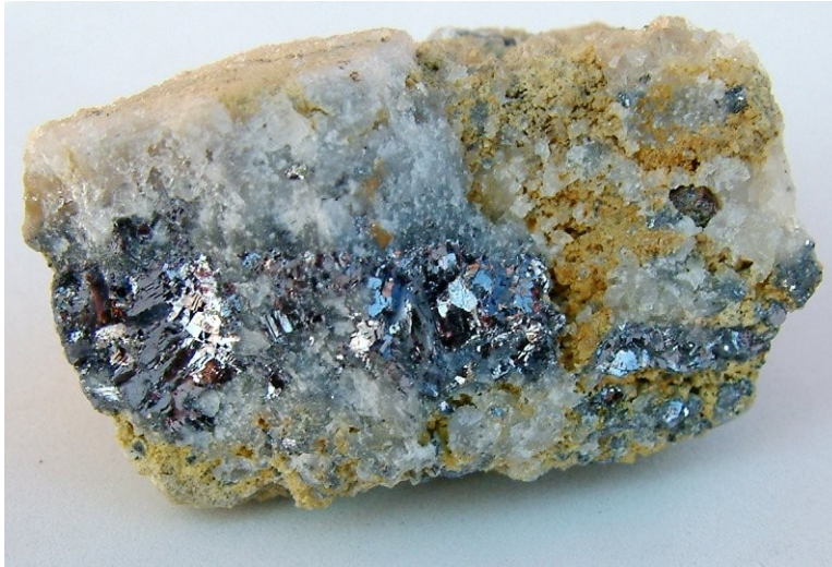
Figure 7.1: Galena mineral (PbS) from Devon, England, UK - The picture shows common galena's appearance in nature (grey color), i.e. as distributed through the quartz vein material (white color). The mineral size is 30mm x 50mm. [256]
