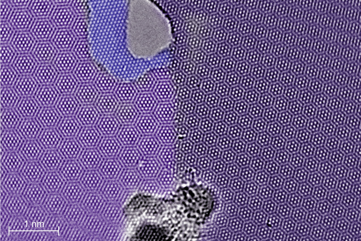
Figure 2.9.: TEM image of CVD grown graphene. A monolayer part of graphene is colored in light blue (top middle). Two twisted bilayer graphene areas with different twist angle are shown in violet and dark blue. Sample grown by Viera Skakalova. TEM image obtained by Simon Kurasch, University of Ulm. The scale bar is 1 nm.
