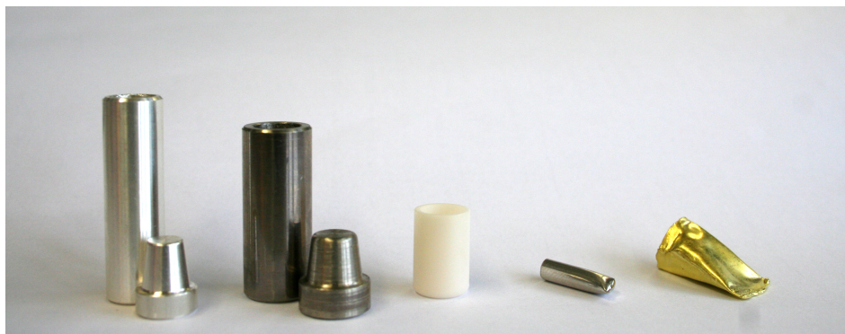
Figure 2.5.: Different types of containers used during experimental part (from left to right: silver, nickel, corundum, platinum, gold).
