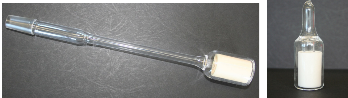
Figure 2.6.: Corundum crucible in the quartz ampoule.
