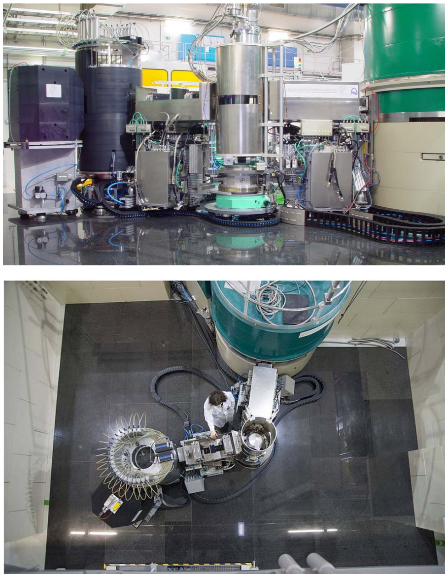
Figure 2.13.: The NRSE-TAS instrument TRISP at the neutron source FRM II, side view (with cryostat) and top view. The monochromator is enclosed in the cyan-colored concrete shielding. Photos from Ref. 20.
