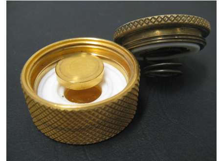
Fig. 16: Sample cell with teflon ring for adjustment of a fixed electrode distance and electrode diameter.
