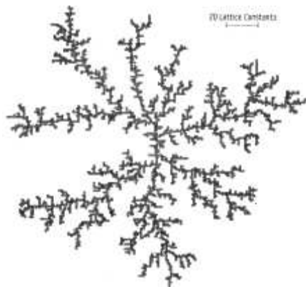
Fig. 19: Fractal cluster from Witten and Sander created by the random aggregation of 3600 particles on a square lattice.
