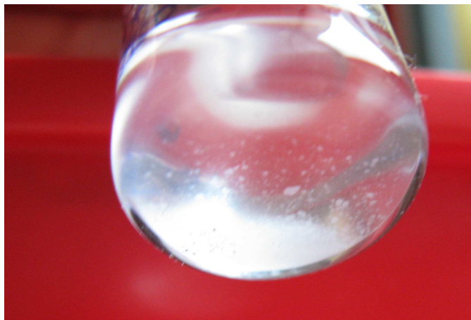
Fig. 40: Sedimented B-PMO (2.8 Vol-%) in 1 M LiOTf / PEG-150 after 2 hours.
