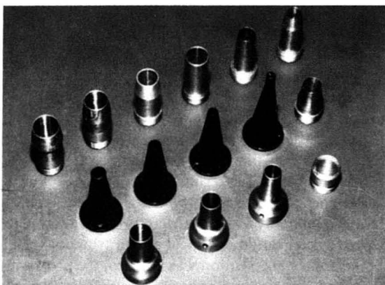
Fig. 9. Photo of different cone sets: Each row was used for a whole measuring session. The cones have decreasing end diameter from left to right. For the two sets in front, the additional cone adapters to the measuring tube are shown at right; the cones of the back row were screwed up directly.
