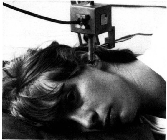
Fig. 11. Photo of the measuring tube: The spark discharge is located in the cubic brass box at top, a condenser microphone with preamplifier is attached below. The measuring tube continues for 75 cm at top of the box (not seen), its lower end is connected to the eardrum via a set of cones with different end diameters to fit best the individual size of ear canals.
