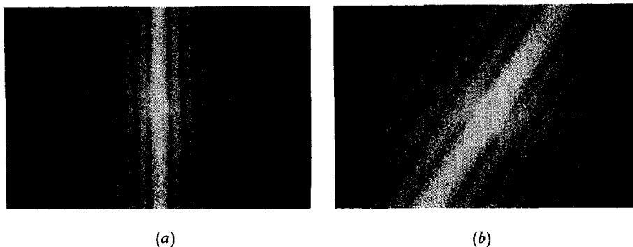
Figure 4. Photographs of the fringes in the Fourier plane of the time average speckle pattern alone (a) 2|\rho_0|=19 \mu\text{m} and (b) 2|\rho_0|=13.4 \mu\text{m} .
