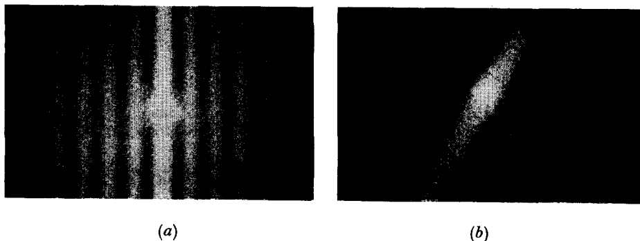
Figure 5. Photographs of the fringes in the Fourier plane of the time average speckle pattern superimposed on that of the stationary object (a) 2|\rho_0|=19 \mu\text{m} , (b) 2|\rho_0|=13.4 \mu\text{m} .
