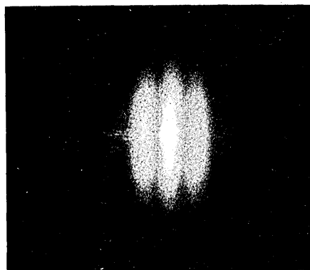
Fig. 10. Example of the fringes in the FDP obtained from a time-average speckle pattern recorded in the Fourier transform plane of an oscillating quartz.
