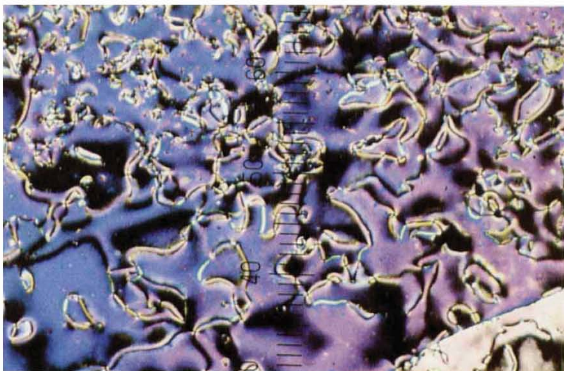
Figure 12. Nematic Schlieren-texture of PET observed between crossed polars in the microscope ( \times 160 ) at 135^{\circ}\text{C} .
