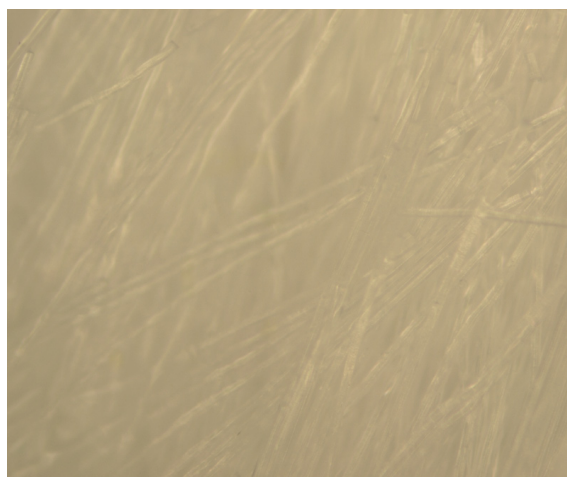
Muffelofen / Probenserie 2 / 100x / Fasern / 750 °C
