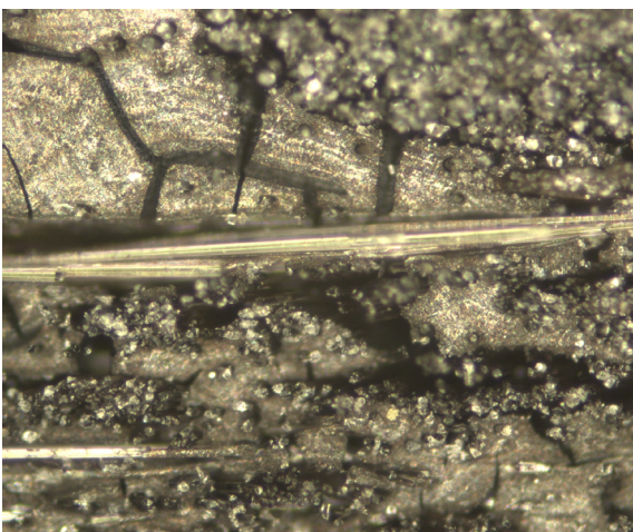
DMA / Probe 4 / 100x / Risse / 450 °C
