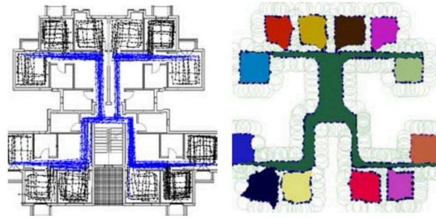
Figure 3.12: Acquired traces (left, blue: corridors, black: rooms) and floor plan (right) resulting from CrowdInside (Alzantot and Youssef, 2012b) (figures adapted)
