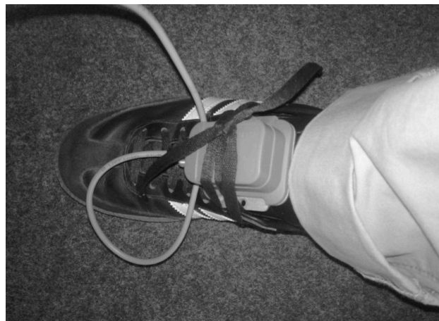
Figure 5.2: Foot-mounted Xsens MTi-G
